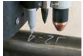
Tube marking/etching: Bend-Tech Dragon obtains the bending information from the Bend-Tech Industrial software to automatically mark and etch bend angle labels, bend locations and rotations.
