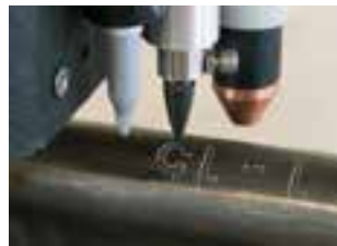
Tube marking/etching: Bend-Tech Dragon obtains the bending information from the Bend-Tech Industrial software to automatically mark and etch bend angle labels, bend locations and rotations.
