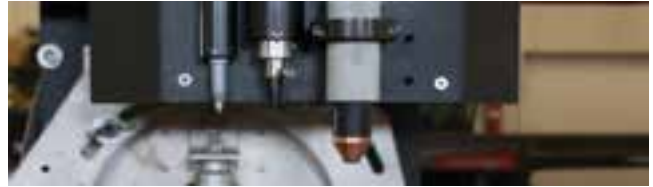
Tool Changer: Machine will switch between marker/etcher/plasma/laser pointer automatically depending on your intended tasks.
